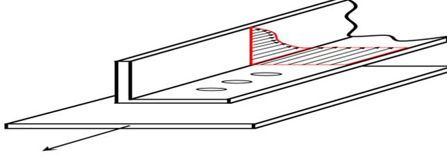
Fig.1 Stress Distribution in unconnected leg due to Shear Lag
